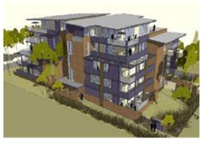
Figure 3.4(e): Building Height. (I) Height controls are based on a typical residential floor to floor height of 3 metres, with a 4.5-0.5 metre allowance for roof articulation and a 1 metre basement projection.
