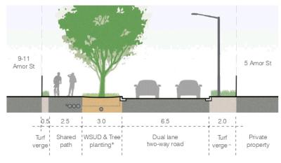
Figure E.16 Wattle Street extension - Section A
