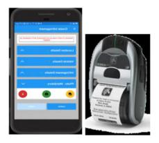
They not only issue and print an infringement, they can take a picture of an offending vehicle, record a conversation with a driver, check back to base data for the vehicle's history of offences and provide a panic button to alert a control room of an emergency situation.
