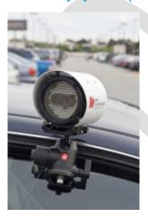
A camera that records vehicles' registration numbers is mounted on vehicles which travel along streets recording the date and time of parked cars. Also known as LPR (licence plate recognition) or ANPR (automatic number plate recognition), they are seldom used for onstreet parking control other than for enforcement.
