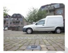
In-ground parking bay sensors, also known as PODs (parking occupancy detection systems), are underground embedded devices which detect the presence of a vehicle in a designated area.
