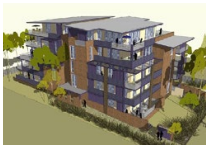
Figure 3.4(e): Building Height. (l) Height controls are based on a typical residential floor to floor height of 3 metres, with a 0.5 metre allowance for roof articulation and a 1 metre basement projection.
