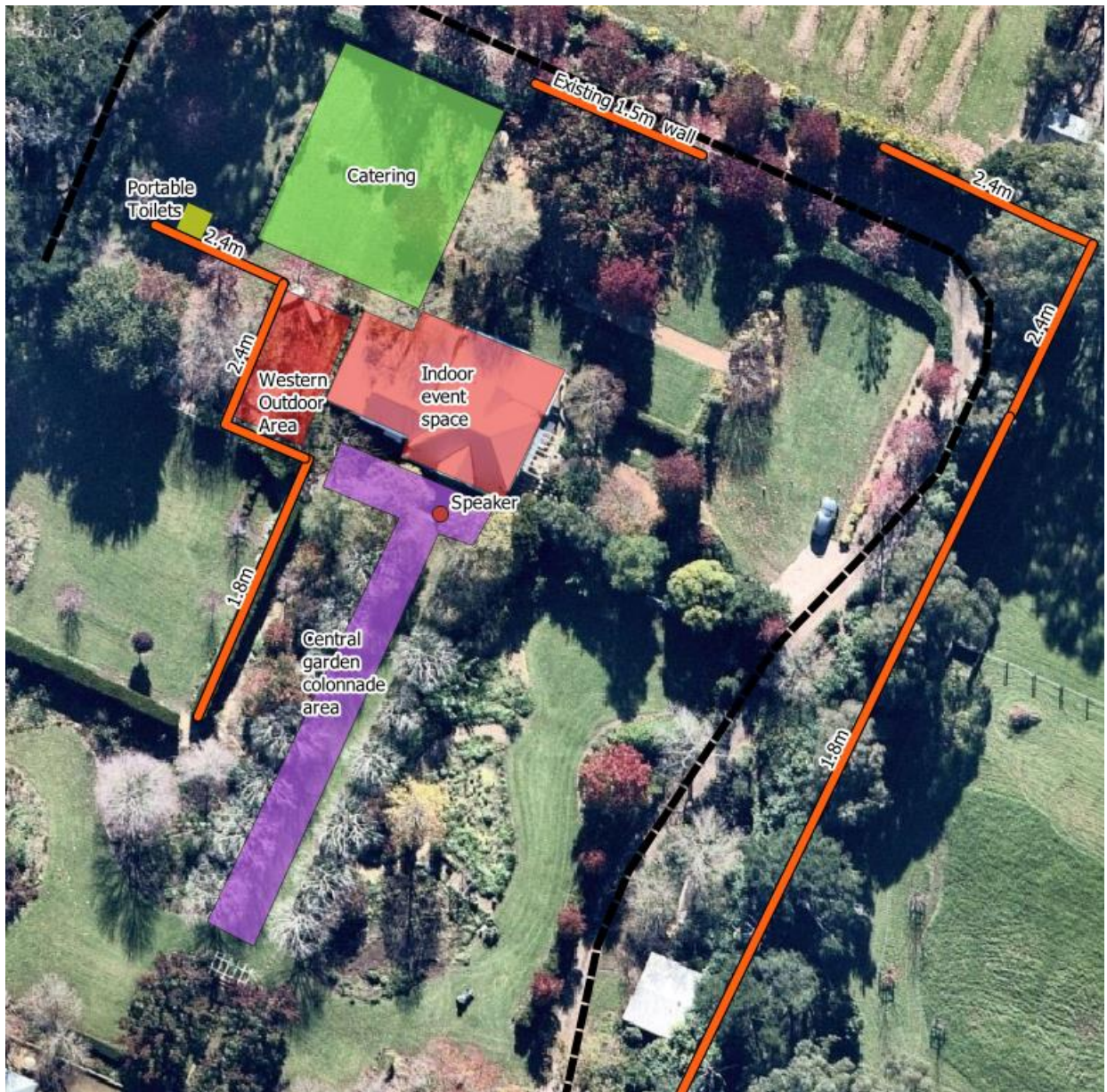
Figure 5-2 Proposed Noise Barriers (The barrier locations are indicative and required to be adjusted for site conditions)
