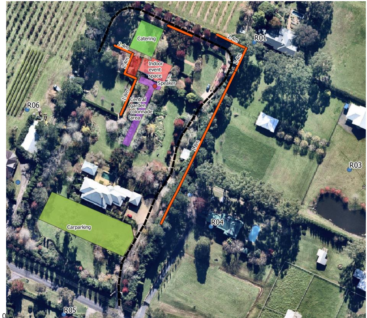
Figure 5-3 Proposed Noise Barriers (The barrier locations are indicative and required to be adjusted for site conditions.)
