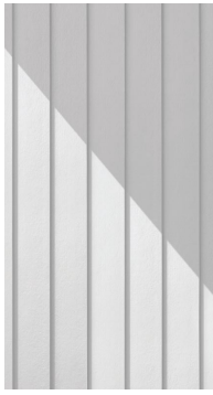
Painted fibre-cement weatherboard cladding typically to upper level external walls.
