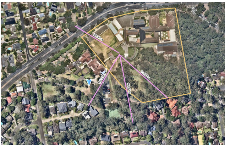
Picture 14 Site boundary shown in yellow, neighbouring low density residential properties between 125-170m away from proposed works. Southern properties shielded by mature canopy coverage indicating negligible acoustic or visual disturbance from proposed works. Properties to the North
