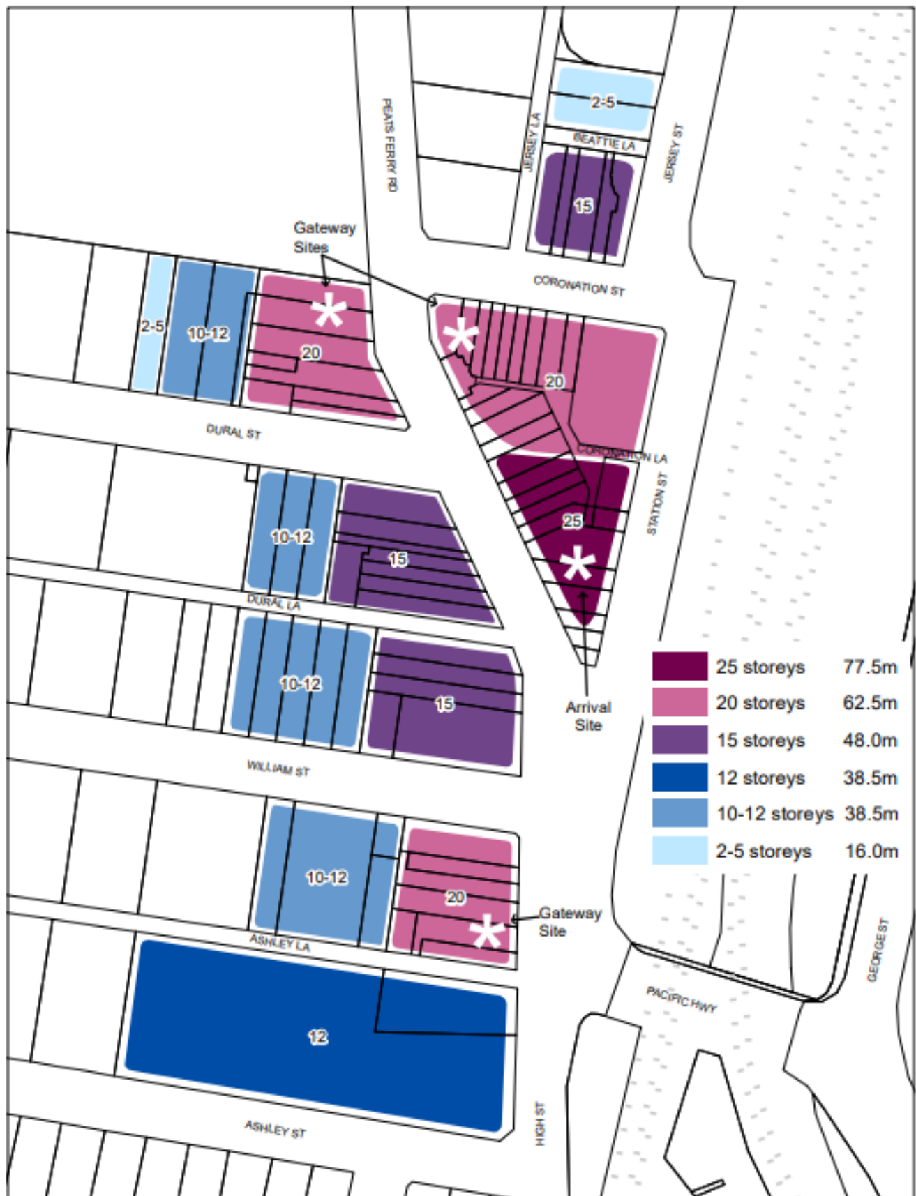
Figure 4.5(i): West Side Precinct - Building Height Plan.
