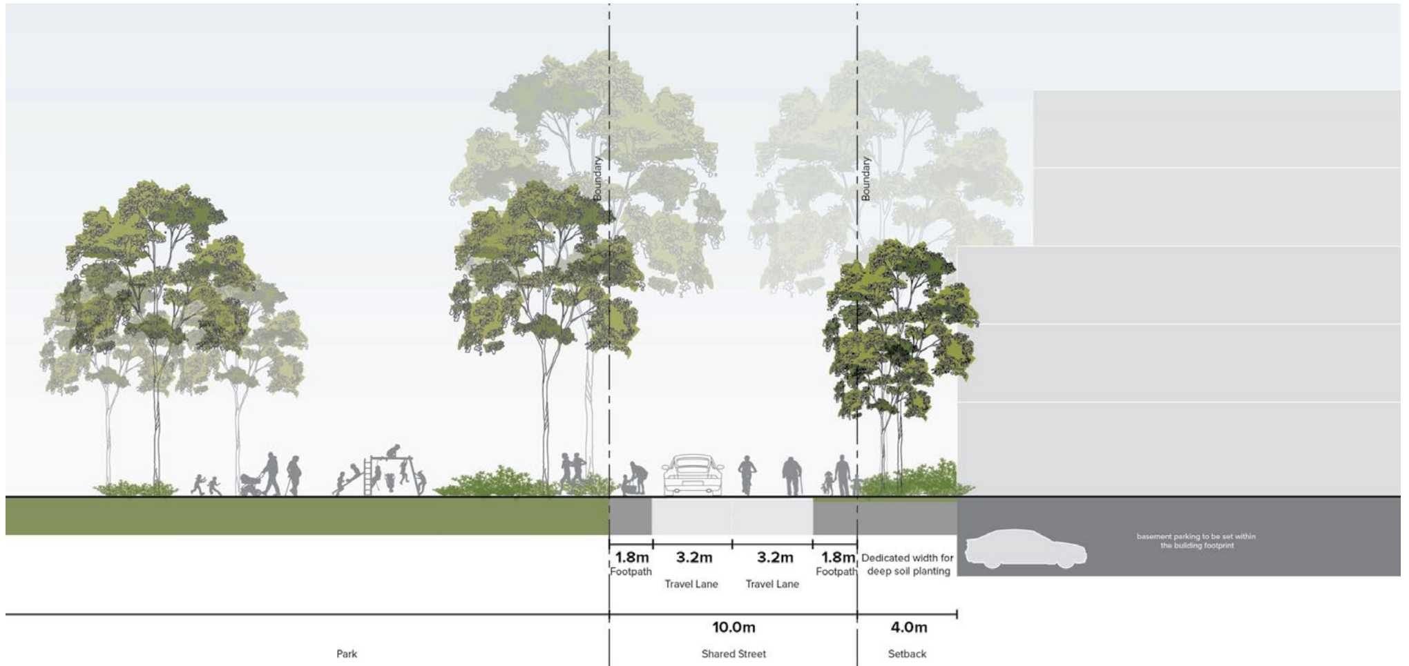
Figure 23: Typical shared street/mews with park interface – indicative street section. Credit: Hatch RobertsDay.
